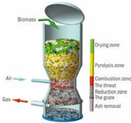
Figure 1: Basic process/design of gasifiers Source: http://www.redeemre.com/downdraft-gasifier.html
